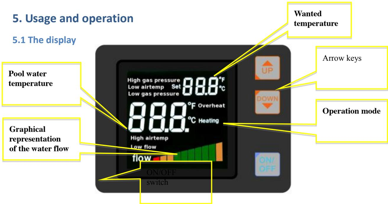
The heat pump can be turned on or off with the ON/OFF button.
